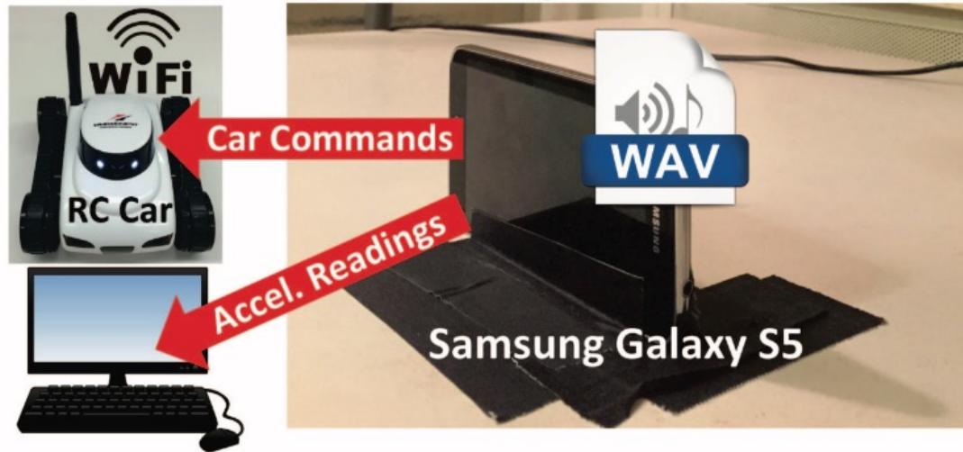
Acoustic Attack on Smartphone Drives RC Car
