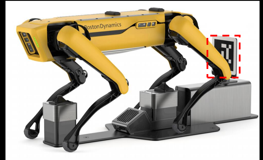
Visual fiducials for precise docking task
